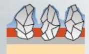
Using a high quality coated abrasive (zirconia with a coating of active grinding additive)
